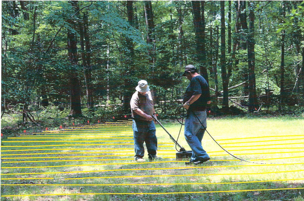
Figure 3. Top: Claude E. "Pete" Petrone operates the electronic equipment associated with the GPR system. Bottom: Bill Hanna (left) and John Imlay operate the 500-MHz antenna south of the walled cemetery.
