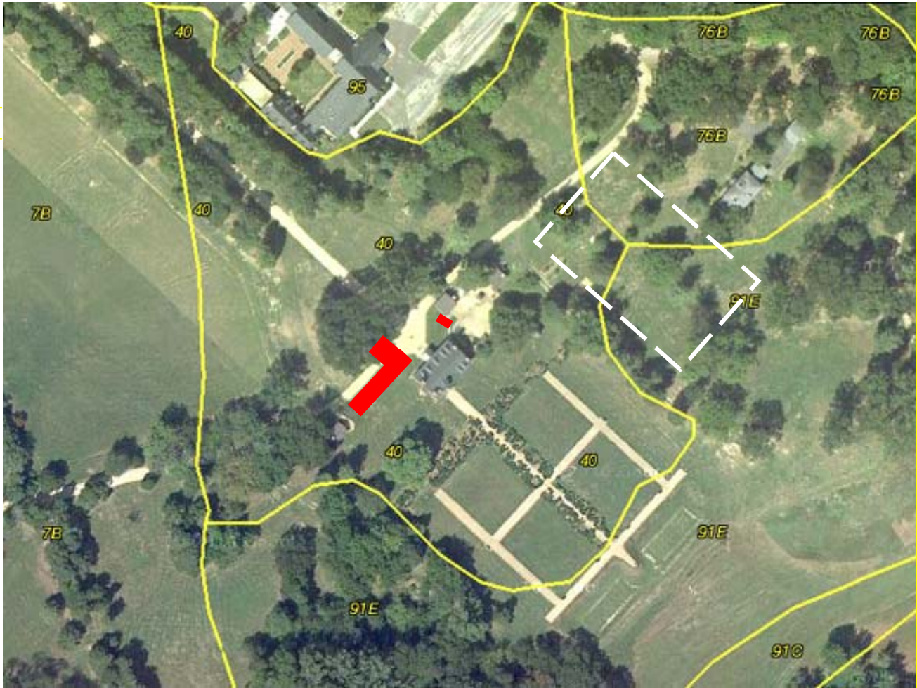
Figure 2. The soil series in the area investigated during 2011 is designated Grist Mill sandy loam (indicated as 40 in the map). Excavation work was done in the areas indicated in red. Soil phosphorus testing was done within area designated by white dashed lines. The surrounding soil series are: Beltsville silt loam (7B); Matapeake silt loam (76B); Sassafras-Marumsco complex with 7% to 15% slopes (91C); Sassafras-Marumsco complex with 25% to 45% slopes; Urban (95). (Detail from California Soil Resource Laboratory 2010).
